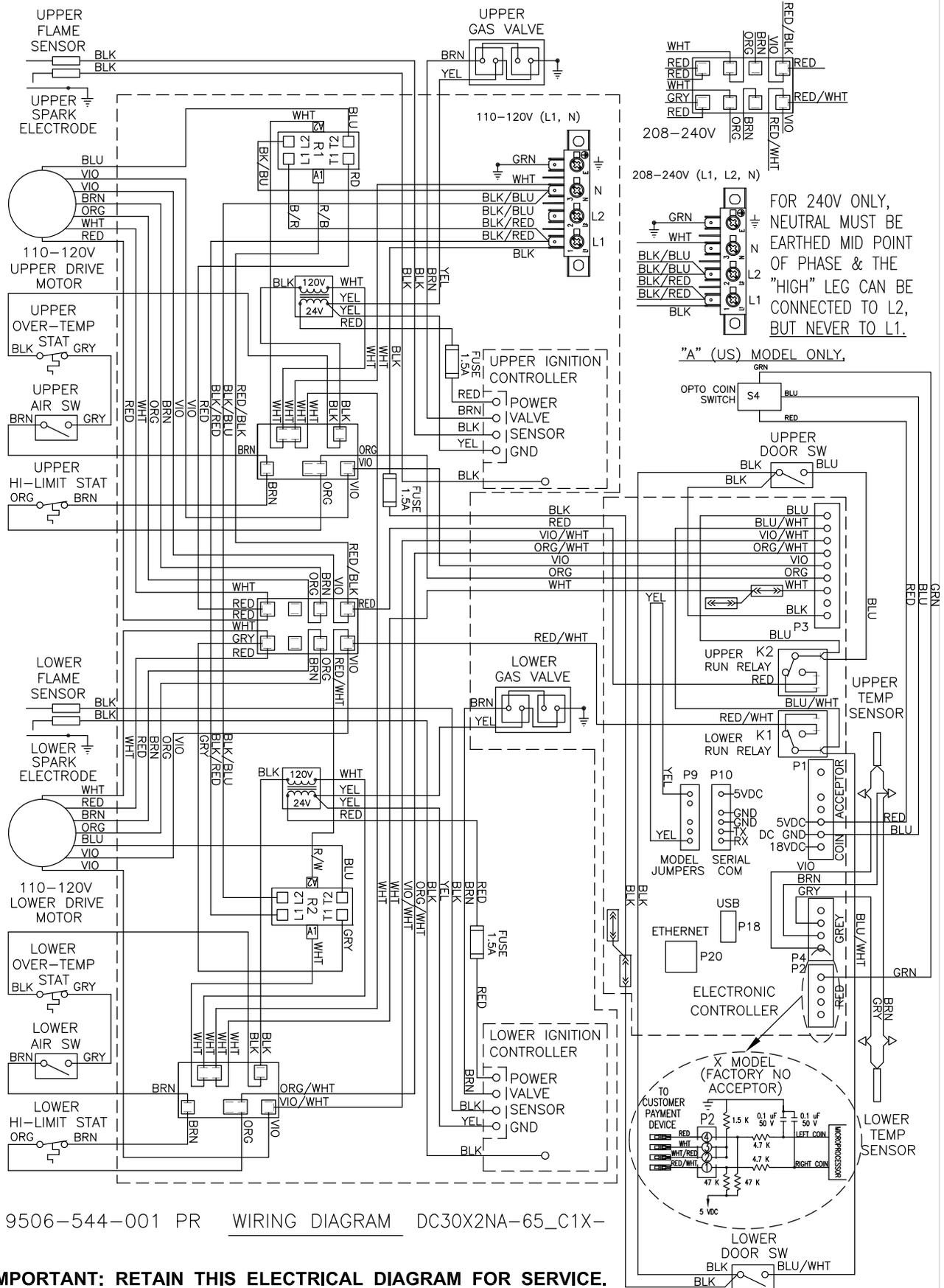
9506-544-001 PR WIRING DIAGRAM DC30X2NA-65\_C1X-
