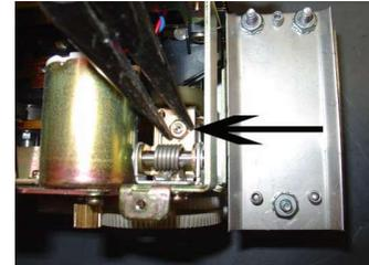
Re-tighten the lock nuts to secure the adjustment. Re-install the reader
