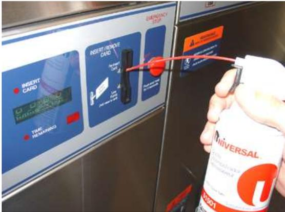
Step 1: Using Canned Air, insert the nozzle into the center of all the readers and give each a quick shot of air.
