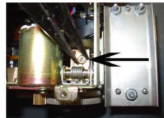
Using a needle nose pliers, loosen the locktight on the nut.
