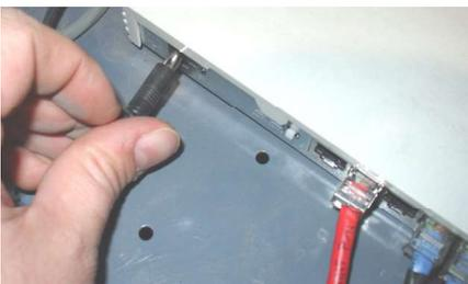
2) If this fails to work, locate the Ethernet switch and disconnect the black power plug that runs to the back of this device. Re-connect the plug to re-establish communications.
