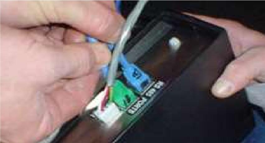
**NOTE:** When running the cables through the machines, keep them away from moving parts, extreme heat sources, and capacitors. Integrated Easy Card™ machines will have the reader cable already connected and located on the back of the Washer or Dryer.
