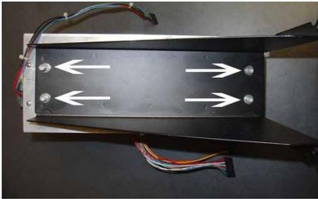
Remove the dispense/ read unit from the shelf assembly by removing the Allen screws on the bottom of the shelf.
