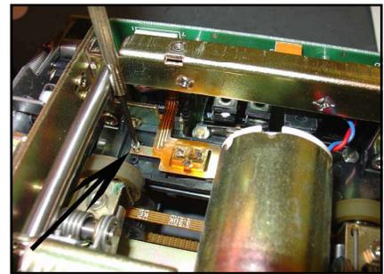
3. Remove the small Phillips screw which holds in the reader head. Check the reader for any foreign objects caught in the reader.
