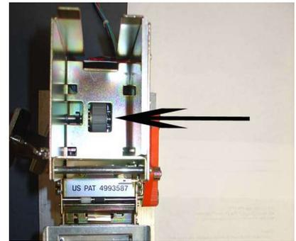
Use the cotton cloth and denatured alcohol to clean the large grey "kicker" wheel in the bottom of the card stacker.
