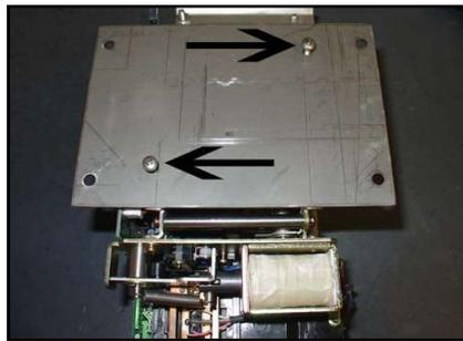
2. Turn the reader over and remove the two Phillips head screws that hold the plate on the bottom of the reader.
