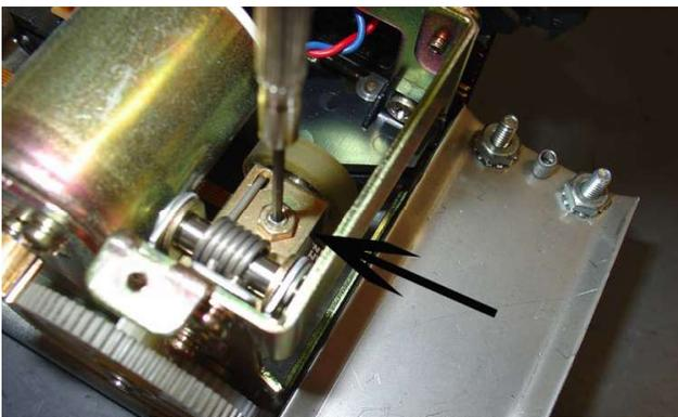
**Step 3:** Using a 1/16 Allen wrench. Adjust the tension. Clockwise will decrease tension, counter-clockwise will increase tension.
