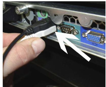
**Step 8)** The modem will be placed on the middle shelf of the Main Cabinet. The 9 pin serial cable will be connected to the only serial port on the back of the Main Server. The power pack will plug into the surge suppressor in the bottom of the cabinet. The phone cable will run from the modem to the modem connection on the battery backup and then the second phone cable will run from the output of the battery backup to a dedicated phone jack.
