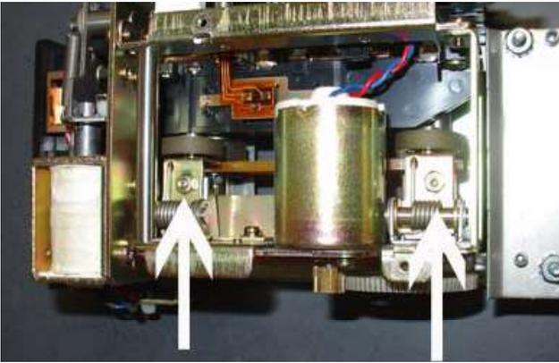
**Step 1:** Locate the lower tension wheel adjustments from the bottom of the reader.
