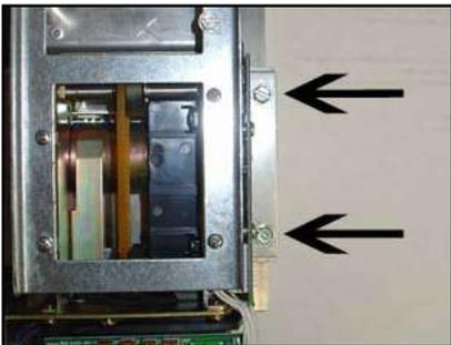
1. Remove the reader from the door by removing the four 5/16 nuts from the sides of the reader plate.
