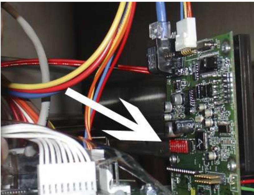
**Step 1A)** When setting Integrated Easy Card™ machines, do not connect the cables to the junction boxes until all readers have been set!
