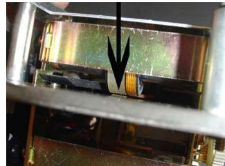
Adjust the back wheels with enough tension that the card can be drawn in yet still slide under the wheels easily. The upper and lower wheels **ABSOLUTELY CANNOT TOUCH**.
