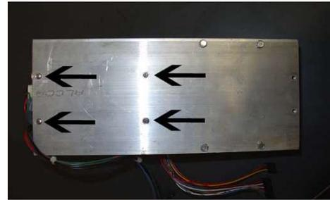
Remove the four Phillips head screws from the bottom of the plate assembly to remove the dispenser.
