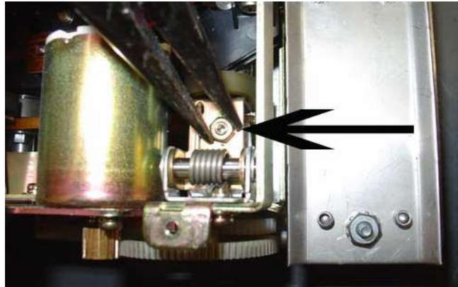
**Step 2:** Using a needle nose pliers, loosen the locktight on the nut.
