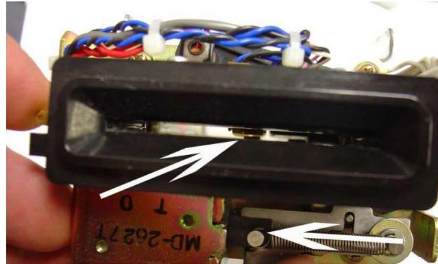
**Step 4:** There should be tension on the card, but the upper and lower wheels **ABSOLUTELY CANNOT TOUCH**.
