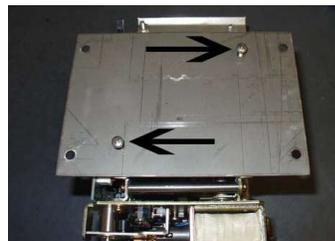
Remove the plate from the bottom of the reader
