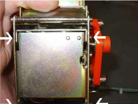
Remove the four Phillips head screws that secure the frontplate. Use compressed air to blow out the inside of the dispenser.
