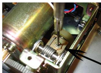
Using a 1/16 Allen wrench. Adjust the tension. Clockwise will decrease tension, counter-clockwise will increase tension.
