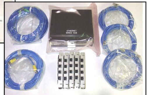
**The network hub assemblies are packaged in with the Easy Card™ large parts box. The single cabinet system will ship with (1) network hub assembly and the dual cabinet system will ship standard with (3) network hub assemblies. More network hub assemblies can be added if the number of pieces exceeds the 32 readers per hub maximum. The assembly includes:**
