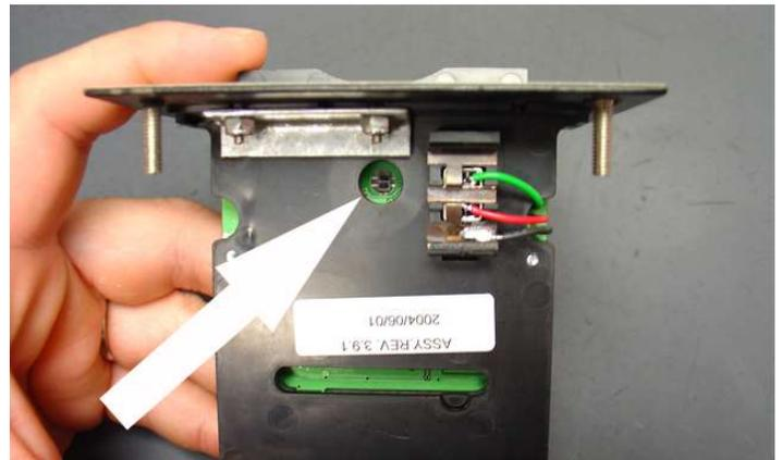
Step 2: This helps to clear lint from in front of the optical sensor.
