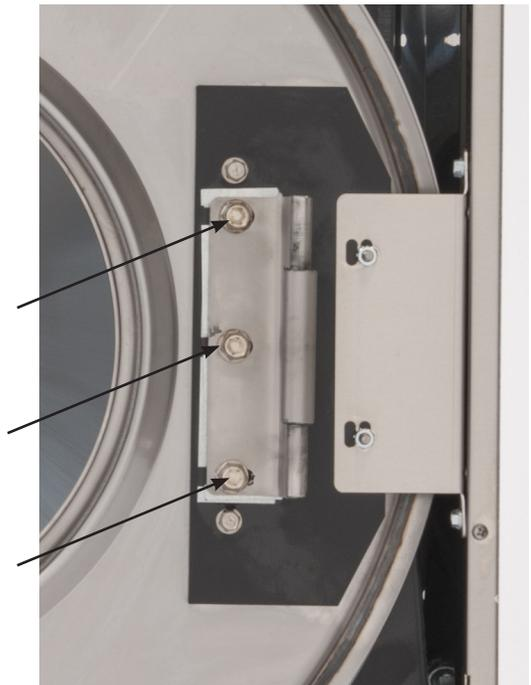
**Step 2:** Remove 3 screws holding door hinge. Shims may be present between hinge and tub front. The number may be increased or decreased to adjust right side door pressure.
