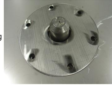
**Step 2:** The tub back assembly should be reattached to the bearing housing with the 6 mounting bolts and torqued according to the torque chart. **NOTE: The bead of silicone that seals each bolt to the tub back. This must be cleaned and replaced upon reassembly (see picture).**
