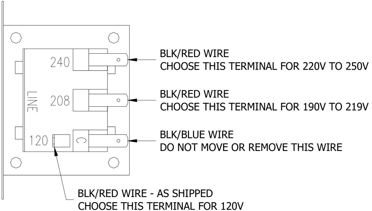
7. Reconnect power to the dryer and test to ensure proper operation; one line voltage to L1, one line voltage to L2 and the earth ground to E.
