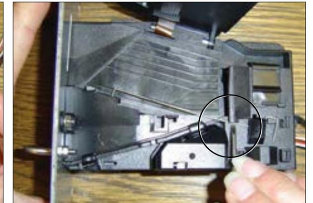
Push the spring below the protrusion by means of a small screw driver. Push the spring lateral to the right until its snaps into its proper position.
