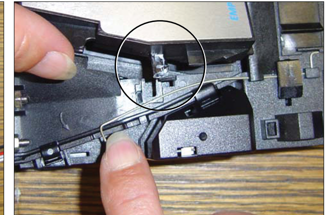
Move spring downwards to free the catch.
