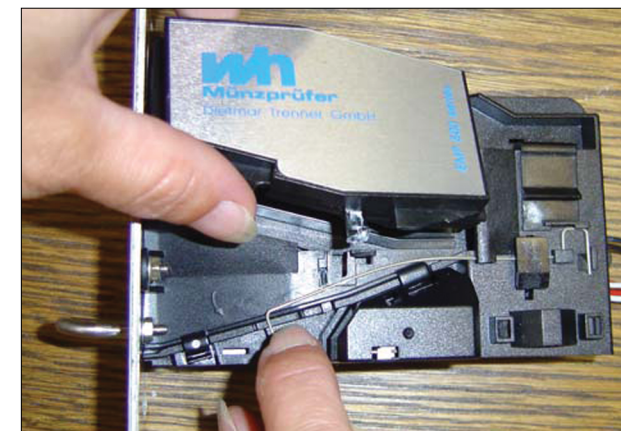
Open the flap of the coin selector.
