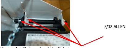
Remove the Motor rod and the Motor.
