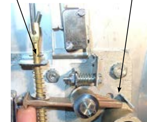
Door lock rod Locking pawl block-
