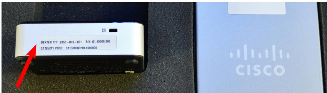
**Note: The Gateway Module and the Cisco Router are matched sets.** Verify that the serial numbers on the gateway and router are the same. This ensures that they are programmed to communicate to each other and to the DexterLive web site. The router is programmed "DHCP enabled". If the location requires that the router needs to be set for a static IP or set up to a different subnet, the information can be found in Section 4 Connecting Cisco Router Internet to the Internet.
