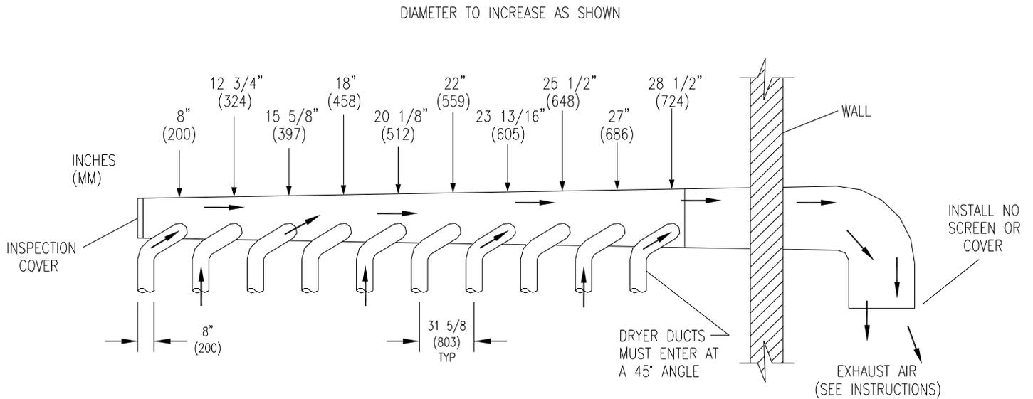
FIGURE 3- Dryer Exhausting Using A Main Discharge Duct.
