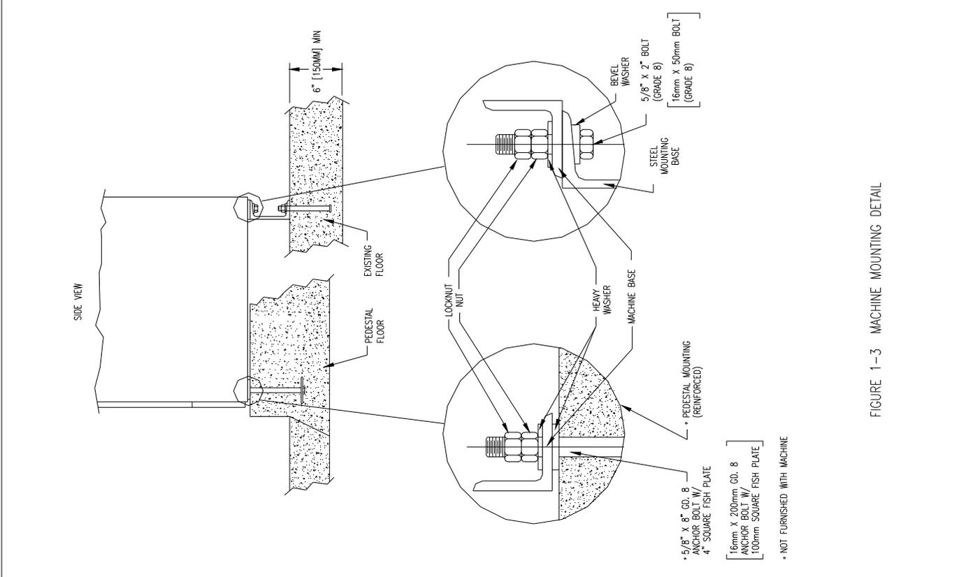
FIGURE 1-3 MACHINE MOUNTING DETAIL
