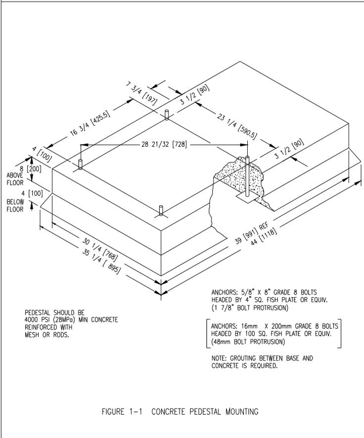
FIGURE 1-1 CONCRETE PEDESTAL MOUNTING
