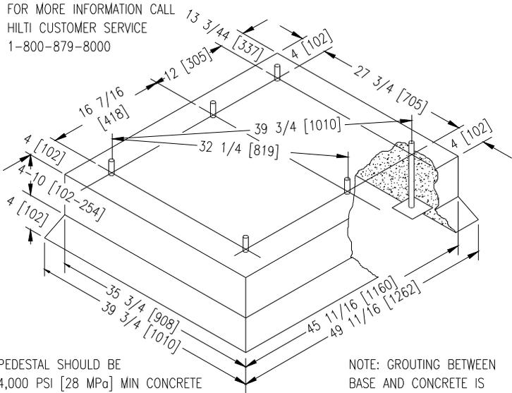
PEDESTAL SHOULD BE 4,000 PSI [28 MPa] MIN CONCRETE REINFORCED WITH MESH OR RODS.
