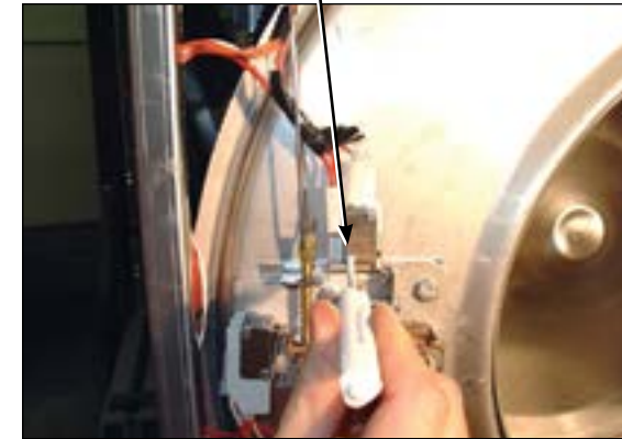
Flat blade screw on door switch latching
