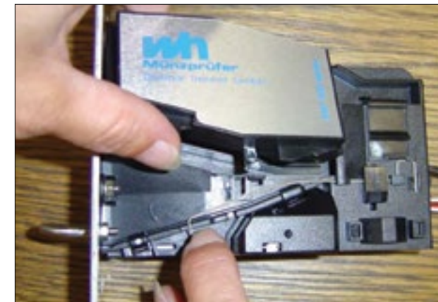
Open the flap of the coin selector.
