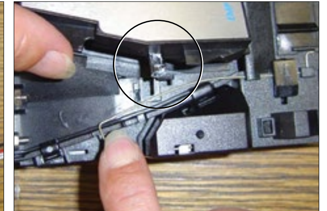
Move spring downwards to free the catch.
