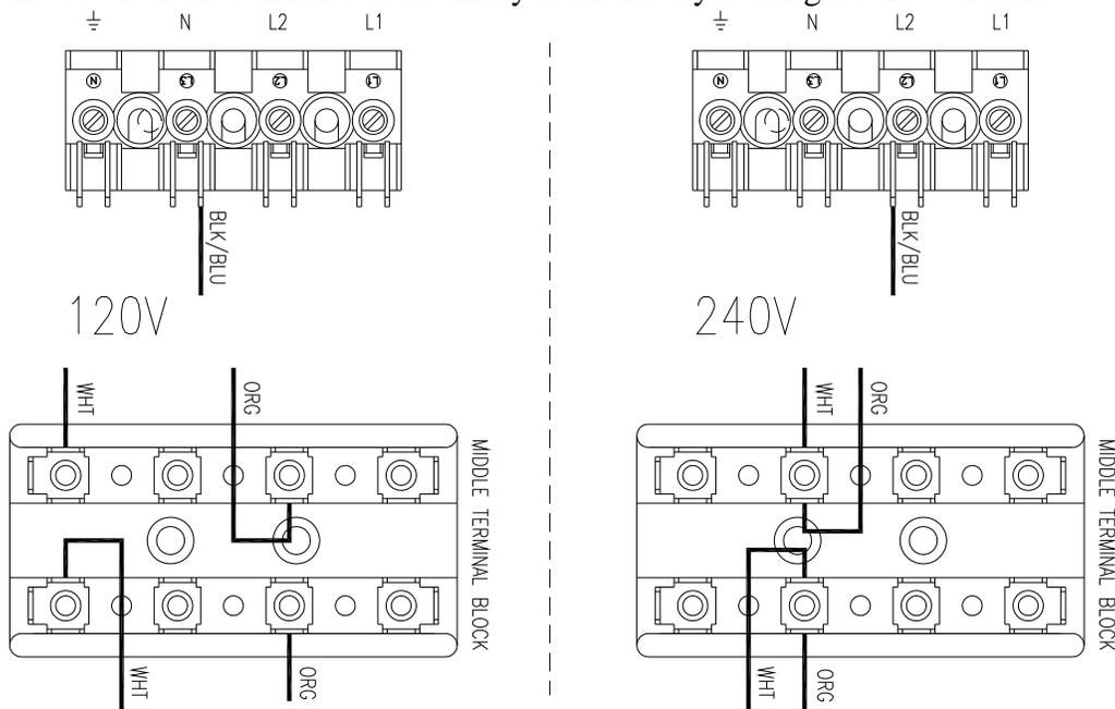
**Figure 6 Dual Voltage Stack Dryer Voltage Conversion**
