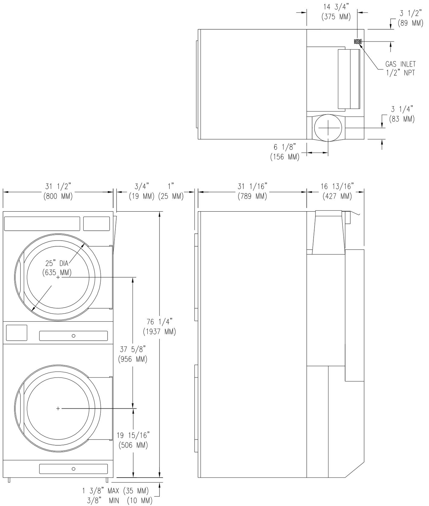
FIGURE 1— Dryer Dimensions – inches (MM)
