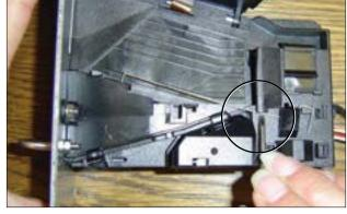
Push the spring below the protrusion by means of a small screw driver.
