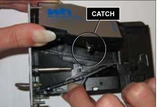
To open the selector move spring downwards to free the catch.
