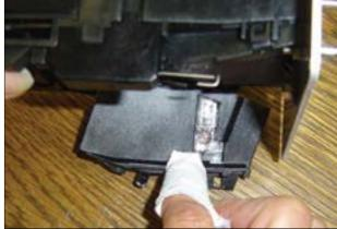
Optical sensors may be cleaned with a soft brush or very carefully with an air spray duster.
