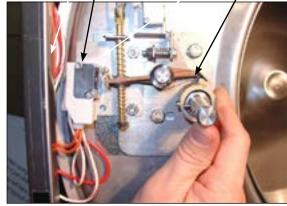
Step 6: The lock stacked switches (piggyback) must be adjusted as door lock gear motor pulls up on door rod and locking pawl is now blocking door cam from turning and is in full up position. The stacked switches (piggyback) have a single actuator arm and it must actuate when single actuator roller wheel rolls to flat side of locking pawl. You will also notice a .040 gap between actuator arm and switch bodies.
