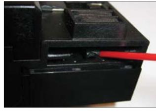
6. Adding the bolt #4036 A bolt can be added to the EMP 500 v4 to reduce attempts of vandalism or to protect the unit from improper
