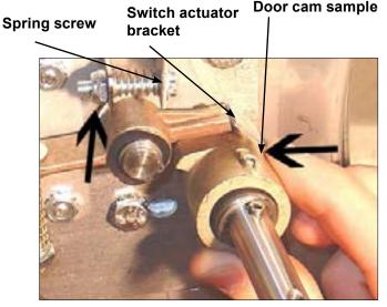
**Step 2:** Tighten spring screw on switch actuator bracket arm until it just clears cam OD. at base of door lock assembly.
