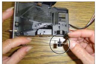
Attach the plastic part to the new spring.
