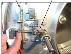
**Step 5:** Check that lock pawl arm swings to cam lobe to lock position.
