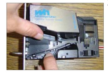
2. Assembly instructions to change a spring Lift the right end of the spring by means of a screw driver.
